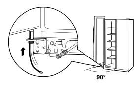
E Set the door on a non-scratching surface with the inside up.
